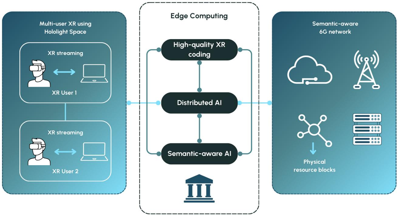
UNITY-6G's "Immersive experience with real-time XR/holographic communications" use case is designed to enable seamless, real-time, multi-user XR collaboration using Hololight Space XR application in industrial environments, supported by a semantic-aware, intelligent 6G network. The system delivers high-quality holographic experiences with low latency, adaptive resource usage, and energy-efficient communication across distributed network layers.
