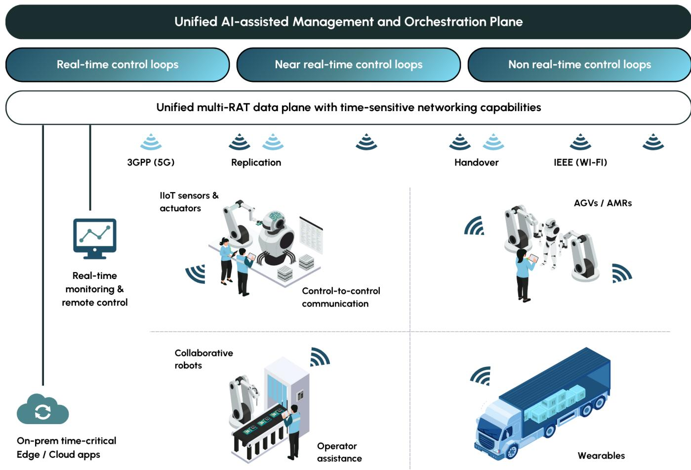
UNITY-6G's "Multi-RAT O-RAN enabled NPN for supporting time sensitive application for Industry 4.0" use case is designed to address the critical need for deterministic, low-latency, and highly reliable communication in automated industrial environments. While current industrial applications often rely on wired Time-Sensitive Networking (TSN), this use case focuses on extending TSN capabilities wirelessly to enhance flexibility and support mobility.
